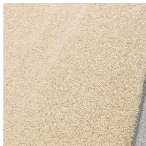
Vehicular Surfacing 2 Coloured Asphalt to Roadway 40mm depth Uticolour Colour: Light Buff Supplier: Tarmac LaFarge Alternative: Tarmac with rolled chippings
